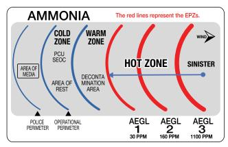
The hot zone starts here at the AEGL-1 line. Since you always have to have the wind at your back when heading towards the area where the leak is, the work areas could end up closer to this leak.
